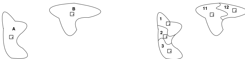
Figure 3.4: Illustration of two regions in the model graph (left), and the typical result after following an over-segmentation process on an image to be recognized (right). This figure also illustrates the centers of gravity of each of the regions. These will be used as a destination point representative of the whole vector from any point of the origin to the destination.
