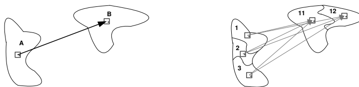
Figure 3.6: Summary of the problem of obtaining the edge attributes between regions A and B in the model graph, knowing the values of the edge attributes in the data graph.
