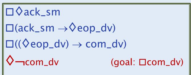
sm = system manager, dv= device ack\_sm: the sm sends an acknowledgment giving permission com\_dv: the dv is in communicating state eop\_dv: the dv sends a signal of end\_of\_process
