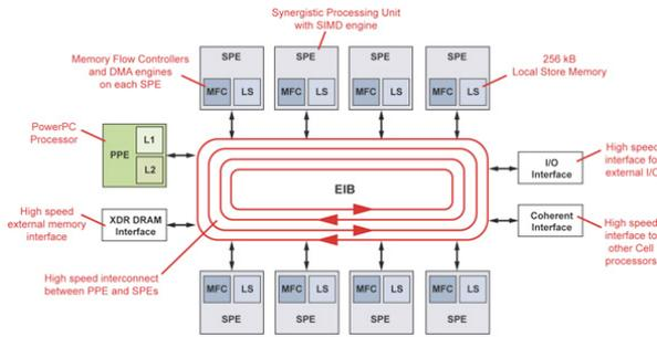
Figure 1: Cell Broadband Engine Architecture.
