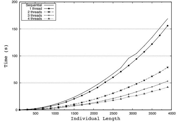
Figure 4: Execution times for sequential and threaded version.
