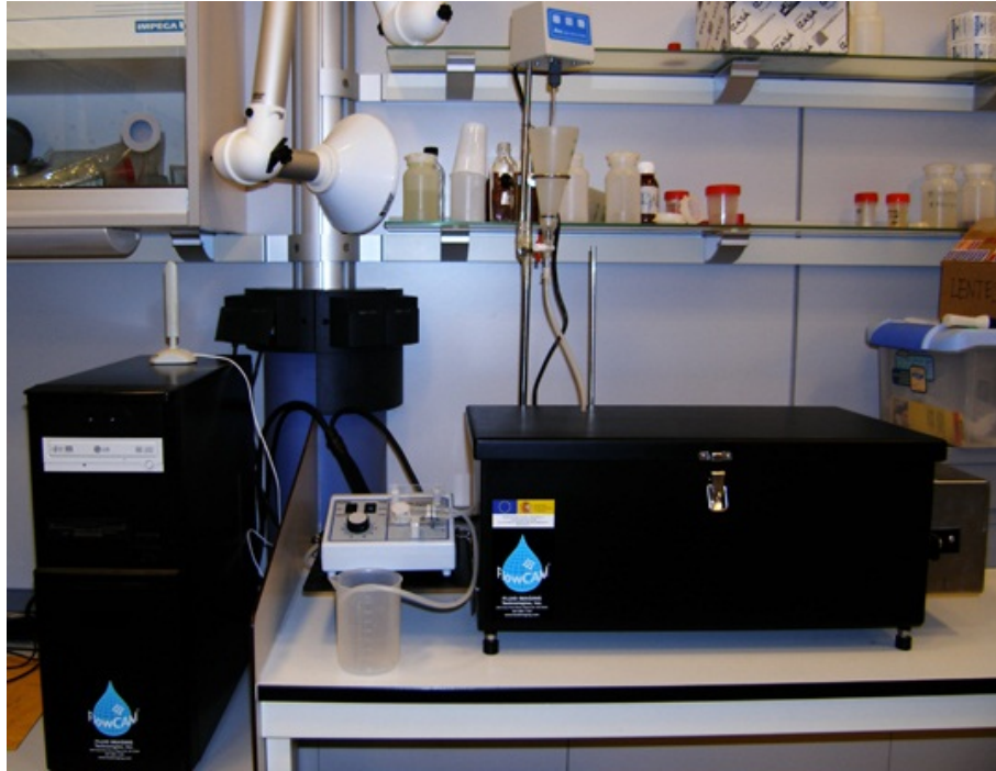
Fig. 1.2. Flowcam, instrument used for phytoplankton digitalization during oceanographic surveys or in laboratories. It is composed of a water plumb, a plastic pipe where the sample goes through and where a digital camera takes several photos per second of the particles in the water sample. Those particles often have sizes inferior to one millimeter. They are later counted and classified using supervised classification methods.
