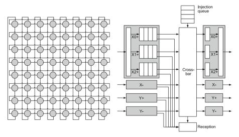
Fig. 6 Left: an 8-ary 2-cube (2D torus with 64 nodes). Right: model of the router simulated by FSIN
