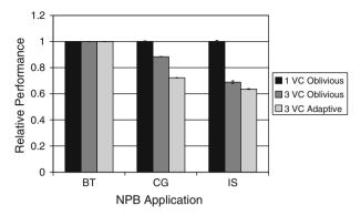
Fig. 7 Effects of using 3 VC per physical link, and of adding adaptivity. Results relative to the base case (Oblivious 1 VC). Average of 10 simulation runs, and 99% confidence intervals
