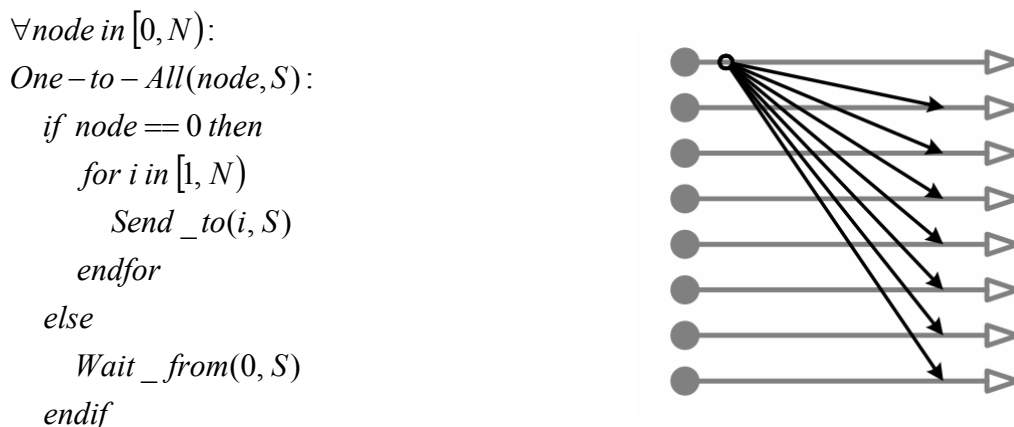
Figure 19. Definitions of the One-to-All pattern algorithmically (left) and graphically (right).
